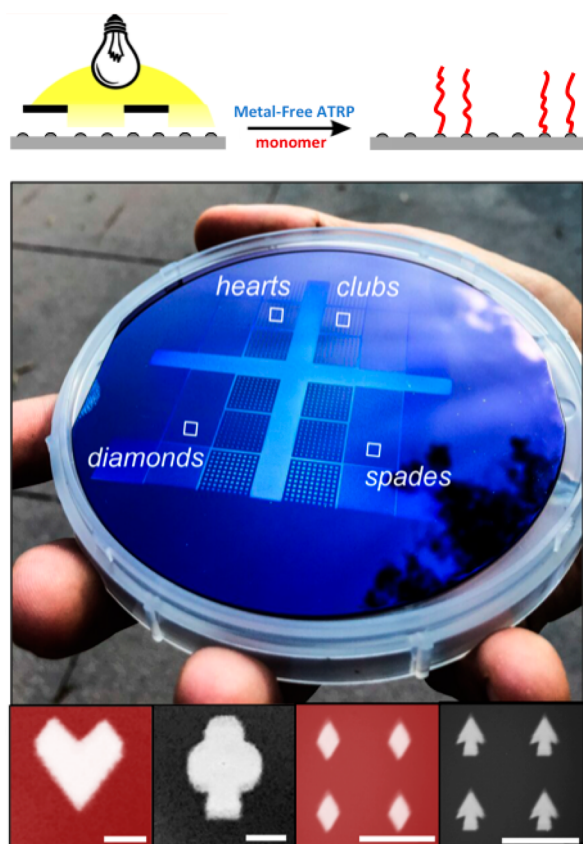
Figure 10. Metal-free SI-ATRP performed on commercial 4 in. silicon wafers using light and a binary photomask to access a range of arbitrary feature shapes and sizes (scale bars are 200 \mu\text{m} ) in one step. Adapted with permission from ref 78.
